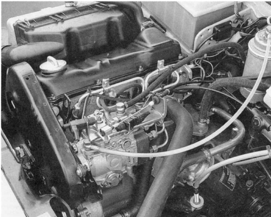
Figure 11.65 VE distributor pump fitted to a 4-cylinder diesel engine
