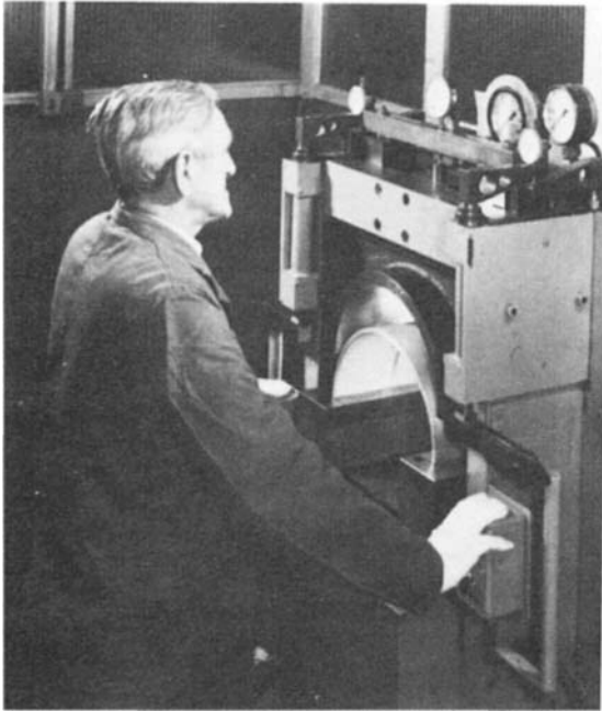
Figure 13.3 Checking peripheral length of a thin shell bearing
