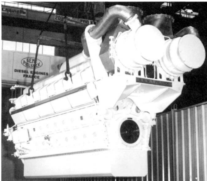
Figure 26.25 SEMT-Pielstick V20-cylinder PA6B STC engine with sequential turbocharging system. A rating of 8100 kW is offered for fast ferry propulsion
