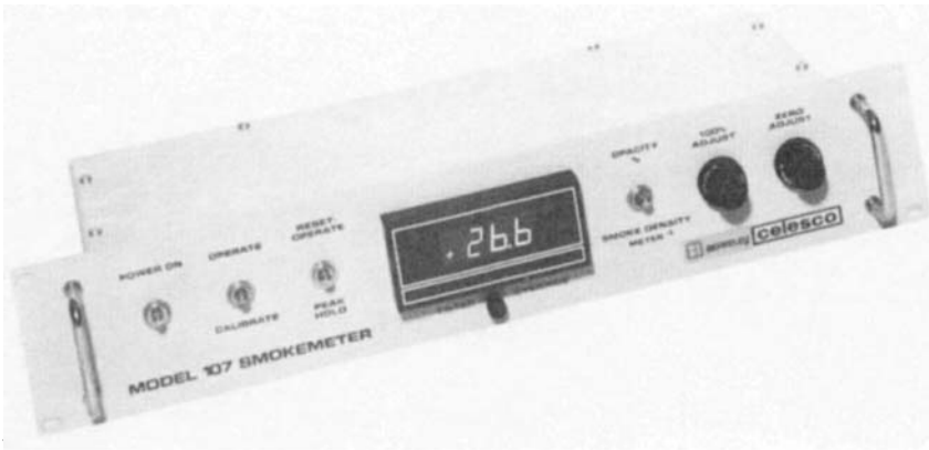
Figure 18.5b Celesco Model 107 Smokemeter output amplifier
