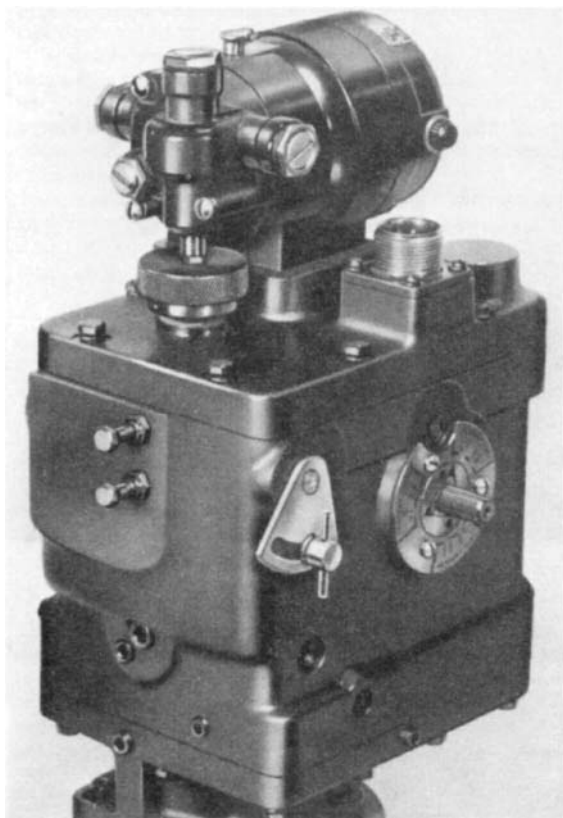
Figure 15.24 A combined electrohydraulic actuator with hydraulic ballhead governor
