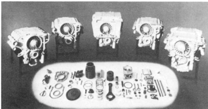
Figure 16.5 Common parts of the engine family FL 413 (Deutz)
