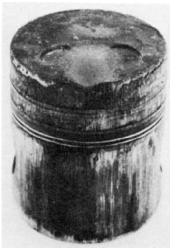
A. Swirl chamber light alloy piston with ‘Torch’ erosion of metal at the point of outflow from the combustion chamber leading to piston seizure
