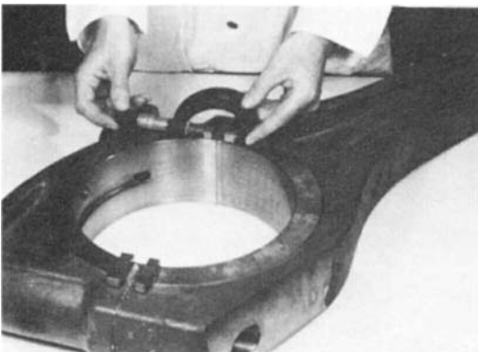
Figure 13.4 Method of checking housing joint face closure
