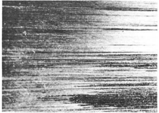
Figure 13.22 Pitted surface caused by electrical discharge
