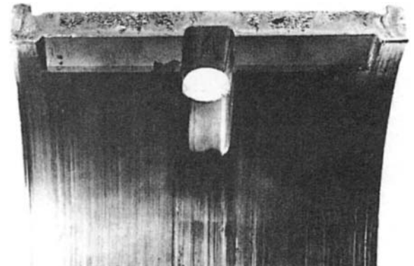
Figure 13.20 Fretting of a bearing joint face due to inadequate bolt load
