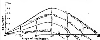
FIG. 14.—Curves of Stability of a Steam Yacht showing effect of variation in height of centre of gravity.
